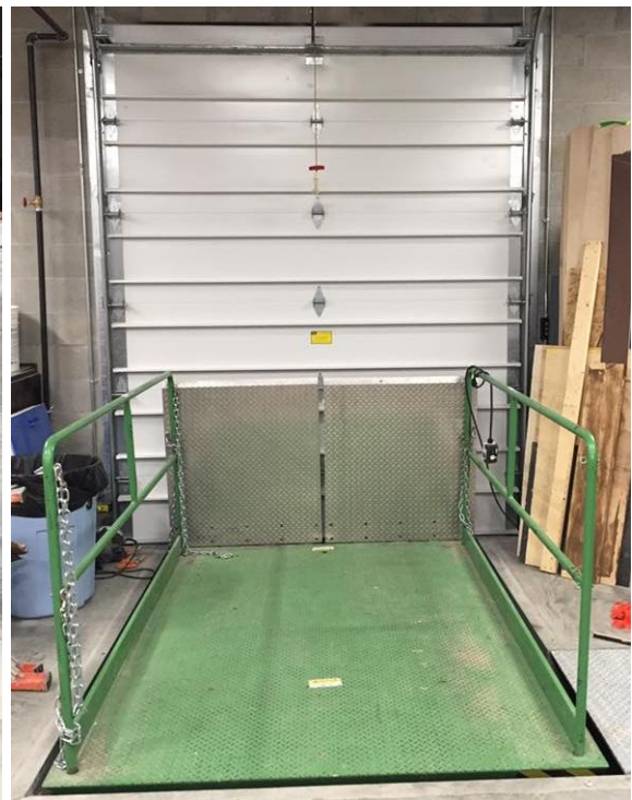
Lift lowered for ground level load-in & interior view. Railings are removeable.
